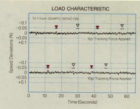
Tracking Force Applied ▼ Tracking Force/Not Applied
