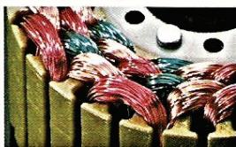
**High-Torque Saturable-Core Motor: The specs are spectacular.** Sansui patents are now pending on this unique and highly effective motor. It is basically a so-called "brushless" design, eliminating physical switching to offer virtually noiseless operation at all times.
