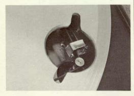
FOUR-POLE HYSTERESIS SYNCHRONOUS MOTOR: The SR-2050C is equipped with a quality 4-pole synchronous motor that quietly maintains constant speeds in the face of fluctuations in line voltage or load. No fine-adjustments of speeds are ever necessary. Special consideration has also been given in the position and method of mounting the motor to obtain an exceptional signal-to-noise ratio.
